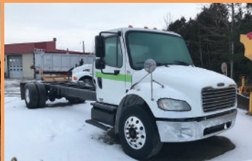
FREIGHTLINER M2-106 2012 , moteur Cummins 8.3 L, 275 hp, essieux 12/23, "Full Lock", Allison
