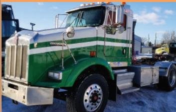
KENWORTH T800 2006 , Caterpillar C15. 475 HP, 18 vitesses, 14X46, suspension air, 506 000 km
